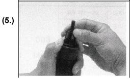
(5.) Push Gun Body's quick releasing ring backward and push part 6 into the Gun Body. Completely release the quick releasing ring to complete the tool assembly.
