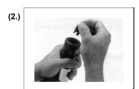
(2.) Insert part 1 into the Gun Body. Rotate part 1 until the slot connects with the Gun Body, shown in the figure to the left.
